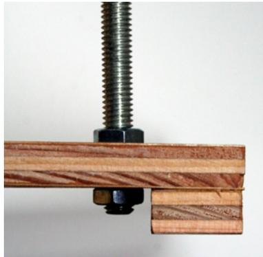
6. Tighten up the top nut against the face of the wood.
