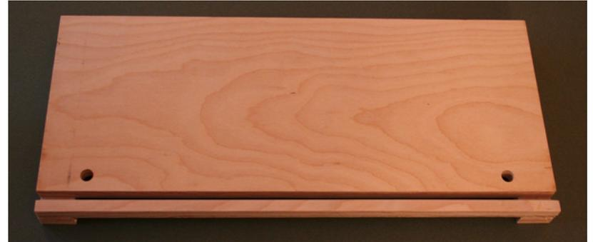
The dimensions of the various pieces of plywood should have left a slot 1/4 inch wide between the bed and the slat in the front.
