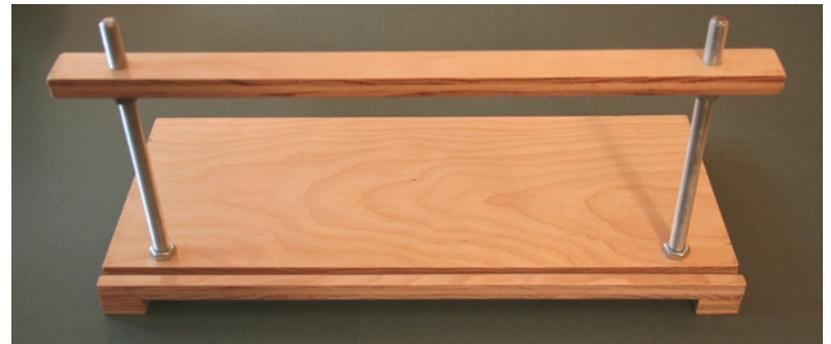
Note: If the crossbar is too tight on the posts to move up and down fairly easily, you can enlarge the holes by drilling them out to 7/16", or even 1/2" diameter.
