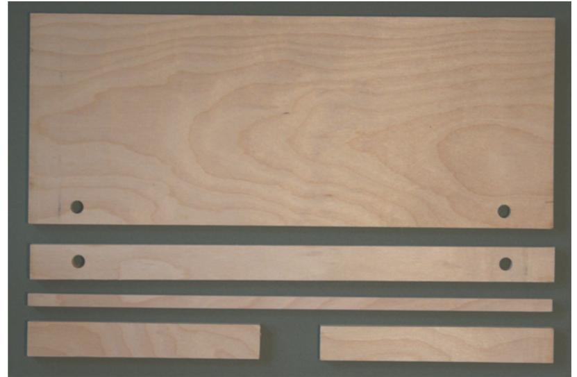
Go over each piece with sandpaper and remove all splinters and sharp edges.
