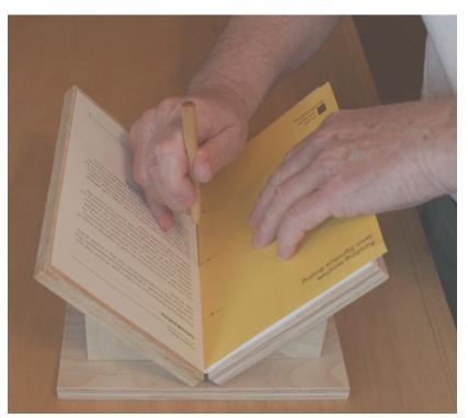
The photograph below shows the punching cradle in use, punching a signature of A-size sheets.
