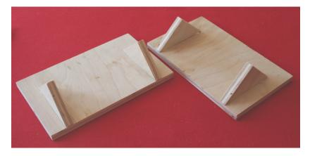
You now have two *side* assemblies. Leave them undisturbed for a couple of hours (or more) for the glue to set up before you go on to the next step.
