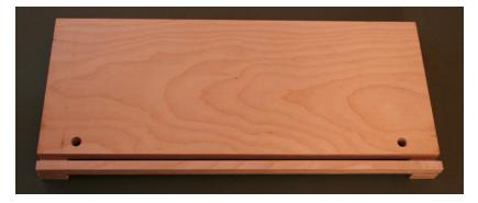
The dimensions of the various pieces of plywood should have left a slot 1/4" wide between the bed and the slat in the front.
