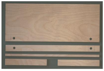
Go over each piece with sandpaper and remove all splinters and sharp edges.
