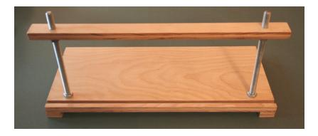
Note: If the crossbar is too tight on the posts to move up and down fairly easily, you can enlarge the holes by drilling them out to 7/16", or even 1/2" diameter.
