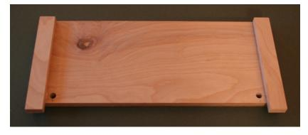
4. Wait a few minutes for the glue to set up a bit, then turn this assembly over so that it is standing on its feet.
